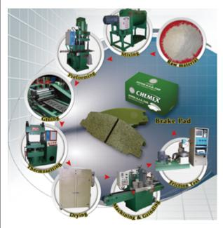
cleaner wheels; increased durability of pad and rotor; and many other advantages. Materials for making these brake pads are non-asbestos, semi-metallic, and ceramic, etc.
